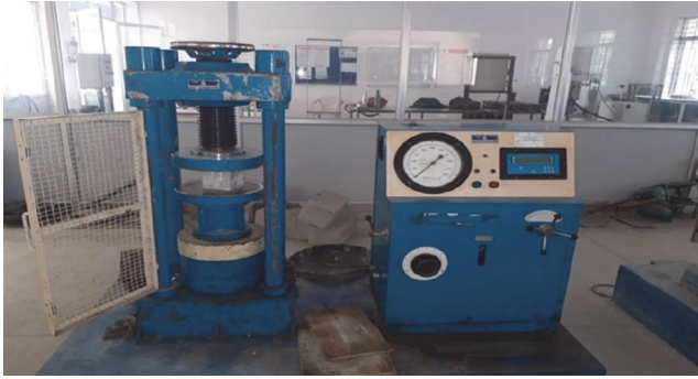
Figure 12. Compressive strength test setup
