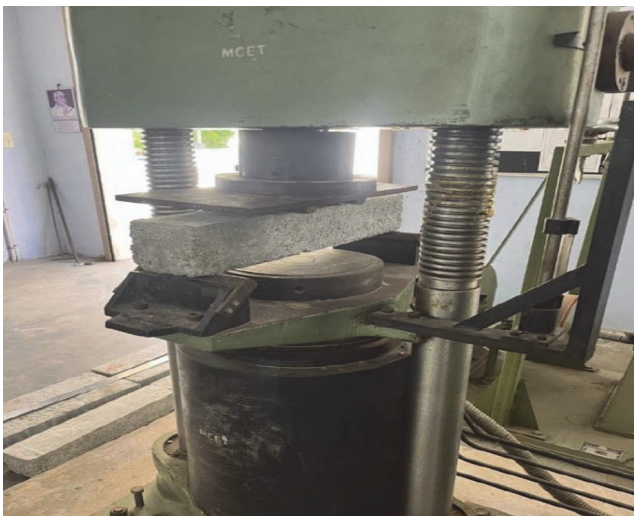
Figure 14. Flexural strength test setup
