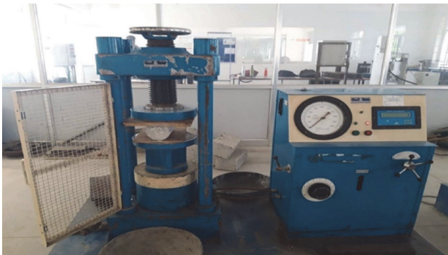
Figure 13. Split tensile strength test setup
